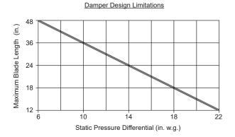
This damper's design at a blade length of 48" has a maximum allowable blade deflection of L / 360 for the static pressure indicated on the chart. At reduced blade lengths, higher static pressure limits can be attained without sacrificing damper operating performance characteristics.
